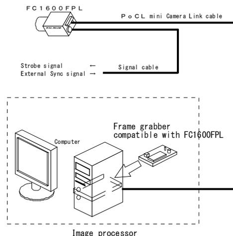
Fig. 4-1 Connection example between camera and peripheral devices
