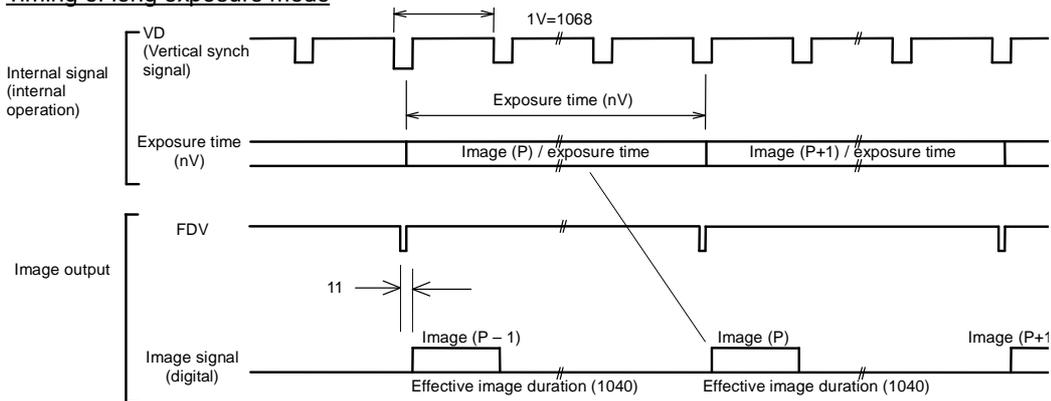
\* The detailed vertical timings of the respective effective image duration are the same as those of “Vertical timing for continuous shutter and without shutter”.
