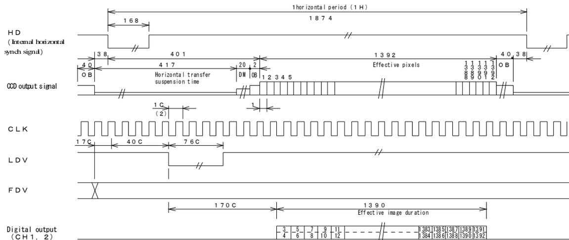
\* Unless otherwise specified, the time unit of the numbers in the horizontal timing chart is pixel CLK (= 1/60.0MHz = 16.7nS), and 1C=1/30.00MHz=33.3ns (CLK output).
