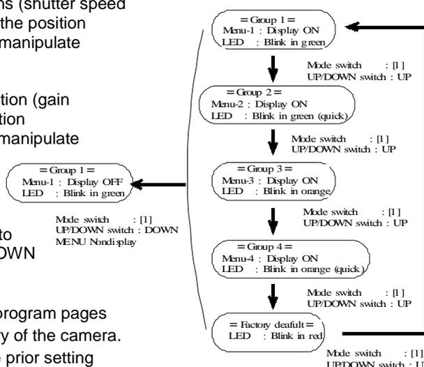
Fig. 6-1 Flowchart of operation mode
