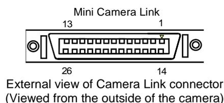
(Note) The pins of Camera Link connector are differently laid out for the camera (upper table) and for the capture board.
