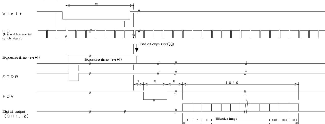
(Note) Strictly speaking, even if the same pulse width of Vinit is applied, the shutter speed differs for the period corresponding to 1H width when the asynchronous shutter operation is executed in the pulse width control mode (indefinite for 1H width).
