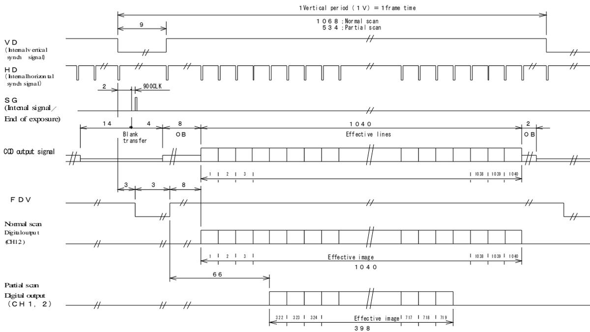
\* Unless otherwise specified, the time unit of the numbers in the vertical timing chart is H(= 1874 PCLK = 1874 x 1/60.0MHz = 31.23μS).
