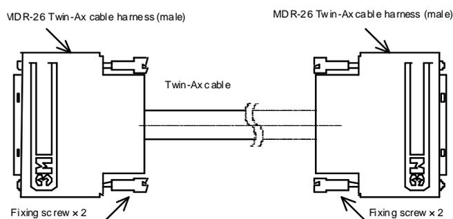
External view of Camera Link cable assembly
