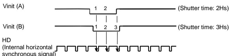
Because of the above reason, consideration must be given to the fact that the exposure time becomes indefinite for the period of 1H shutter speed when a Vinit signal that is not in synchronization with the internal horizontal synchronous signal (HD) is input from the user side. Some of the countermeasures to be taken are as follows:
