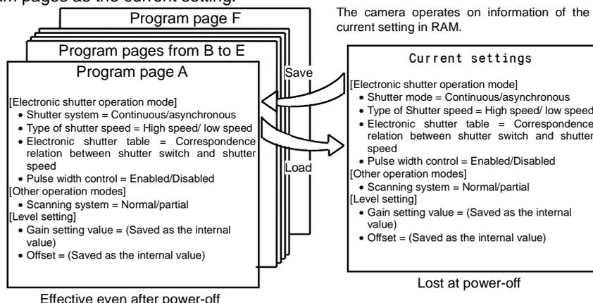
Fig. 6-2 Conceptual diagram of saving and loading operations
