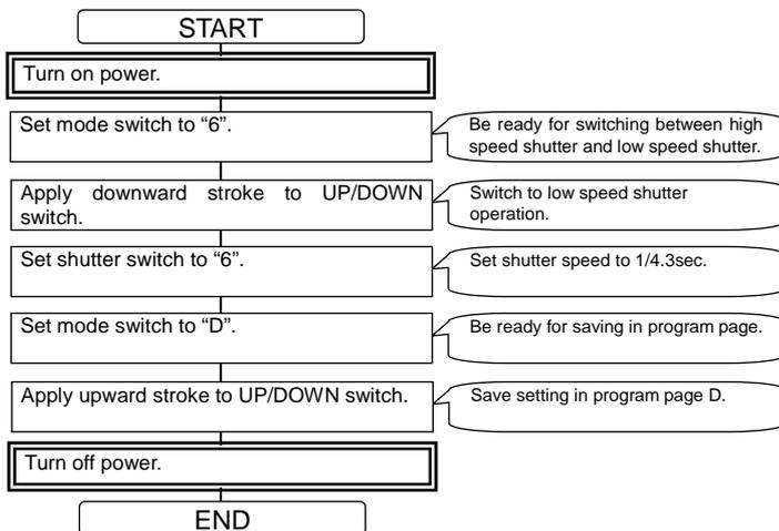
(Example 2) This is the procedure for use in continuous/ low speed shutter operation (1/4.3 sec.)
