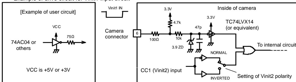
\* The Vinit signal should not include unnecessary noise components such as chattering.
