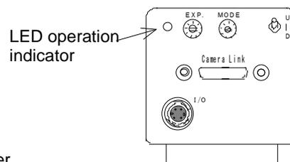
Red LED lights up in response to trigger signal input (Vinit).
