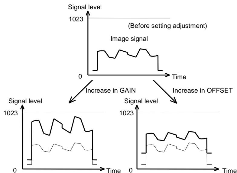
Fig. 5-2 Conceptual diagram of gain and offset levels
